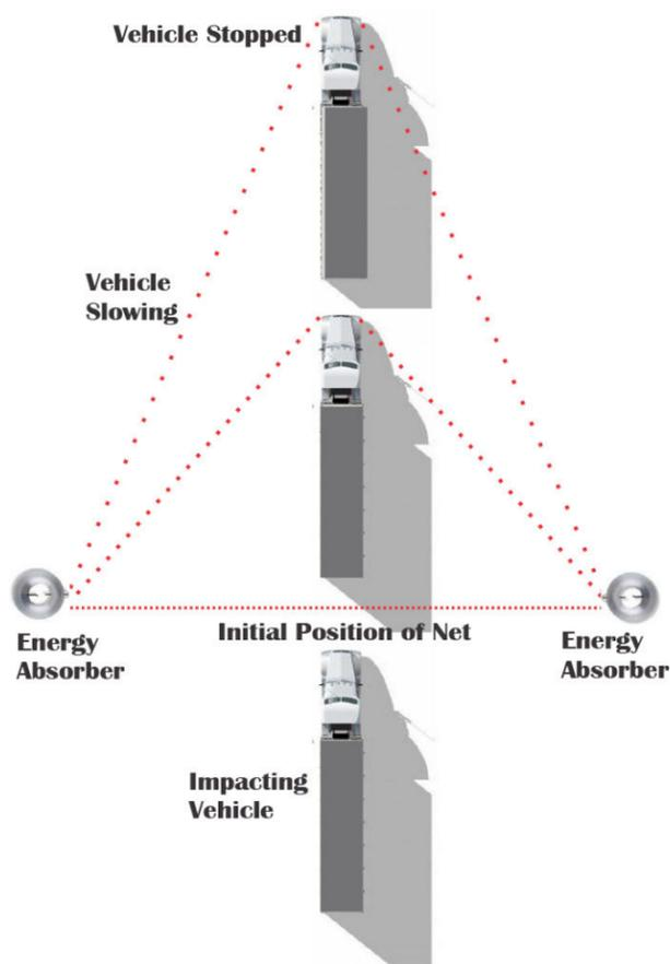
The Dragnet Truck Escape System is comprised of a series of nets set up along a truck escape ramp. The array of nets is arranged in such a manner so as to stop the vehicle in the distance allowed, while minimizing the deceleration forces. These nets, which are made of aircraft cable, can have one or two energy absorbers connected on each side.
