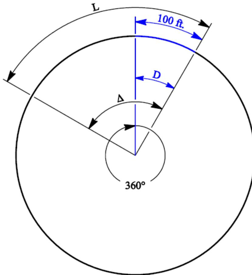
**Figure D-3. Degree of curvature.**
