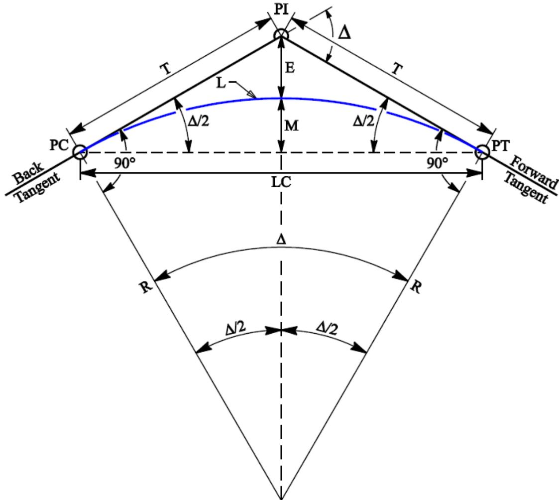
**Figure D-2. Circular curve components.**
