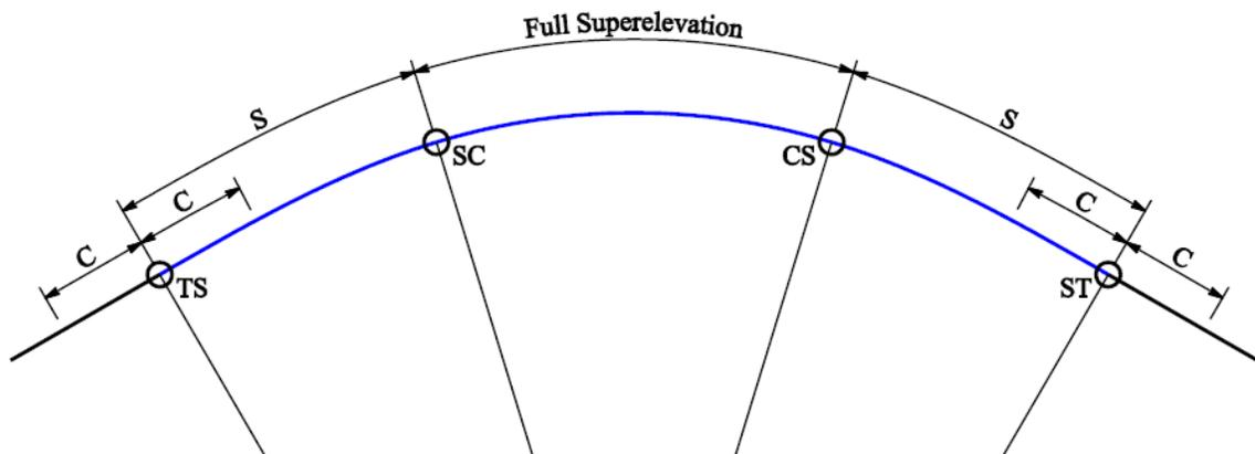
**Figure D-9. Superelevation on a spiral/circular curve combination.**
