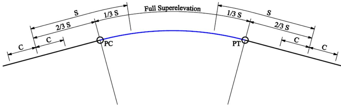
**Figure D-8. Superelevation on a circular curve.**
