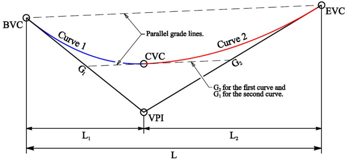
Figure D-12. Unsymmetrical vertical curve.
