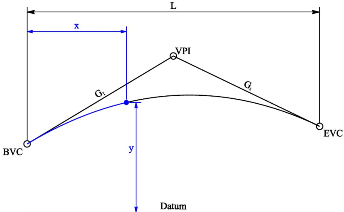
**Figure D-11. Point on a vertical curve.**
