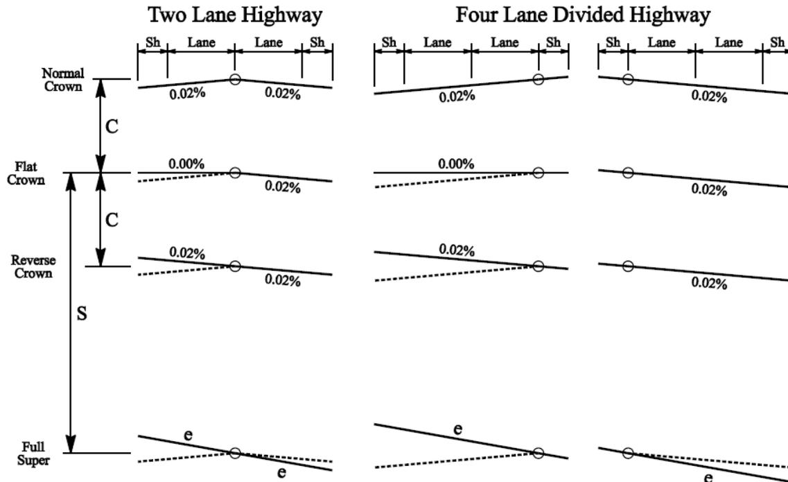
Figure D-7. Superlevation rotation.
