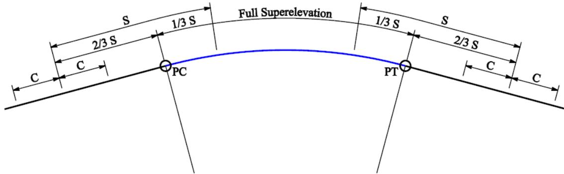
**Figure D-8. Superelevation on a circular curve.**
