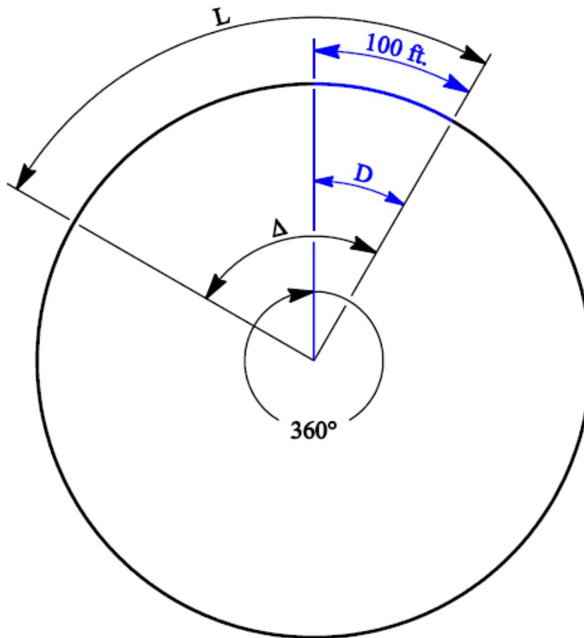
**Figure D-3. Degree of curvature.**
