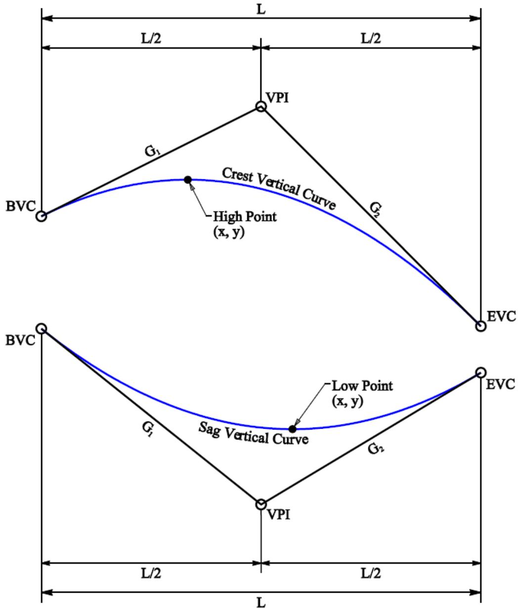
Figure D-10. Crest and sag vertical curves.
