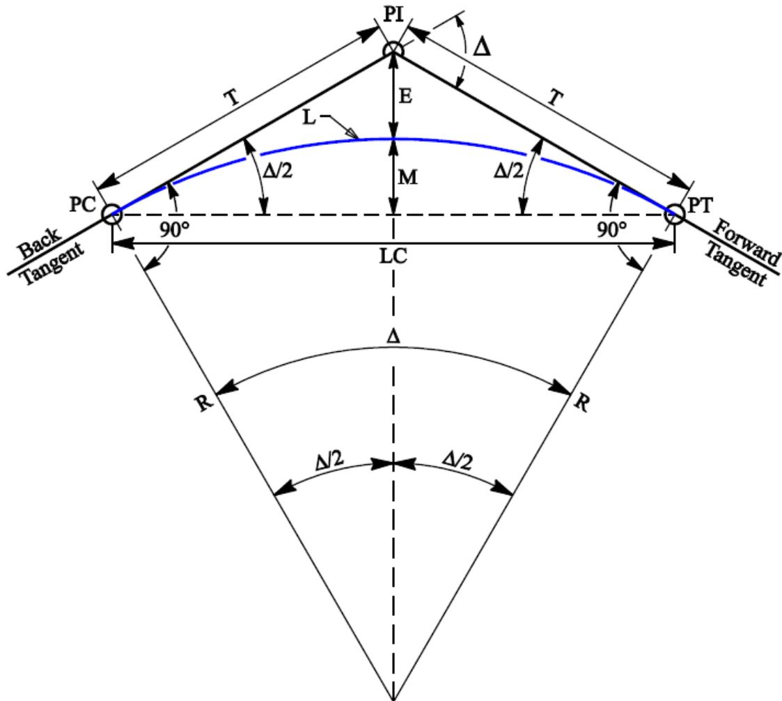
**Figure D-2. Circular curve components.**
