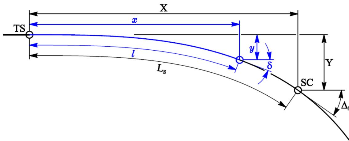
**Figure D-6. Point on a spiral curve.**
