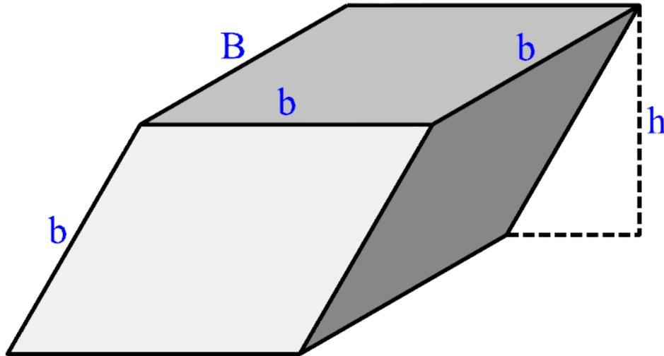
*Figure F-4. An equal-sided oblique prism.*
