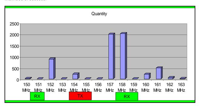
This second chart depicts the available frequencies sorted in 1 MHz increments. The red and green markings indicate the proposed VHF re-banding plan. Clearly, the Ritter Plan negatively impacts the process. The final band-plan will be based on the distribution of frequencies that remain after the sifting process.
