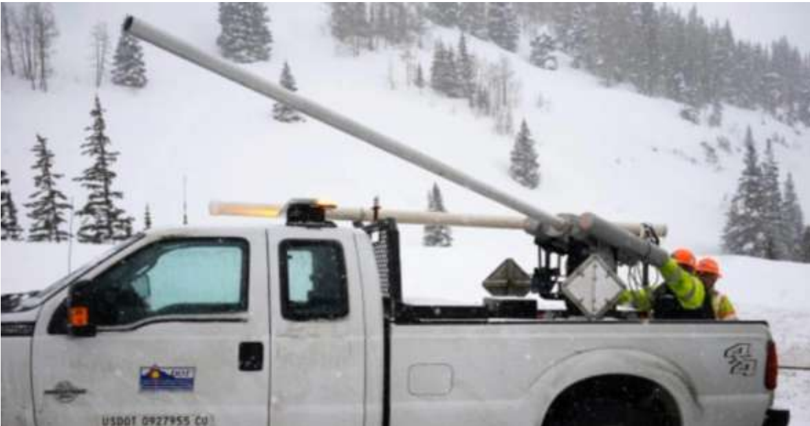
Figure 10. An Avalauncher® being operated by Colorado DOT personnel from a vehicle mounted platform.
