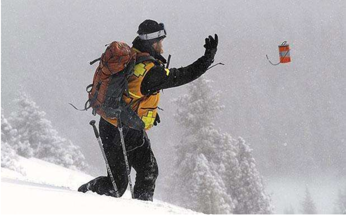
Figure 2. An explosive hand charge being thrown into an avalanche-starting zone at the Copper Mountain ski area, Colorado.
