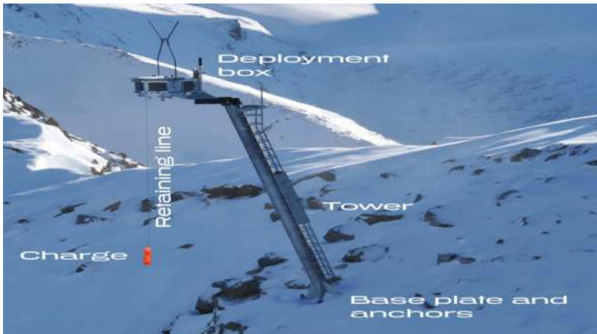
Figure 5. A remotely operable explosive deploying technology, by Wyssen Avalanche Control, in an avalanche-starting zone in the Alps.
