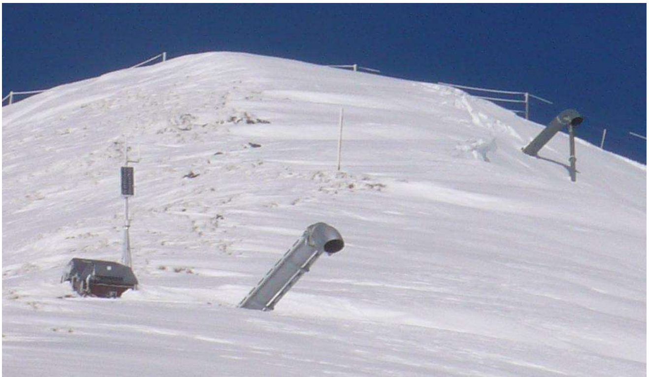
Figure 15. A Colorado DOT deployment of multiple modern GAZEX®.
