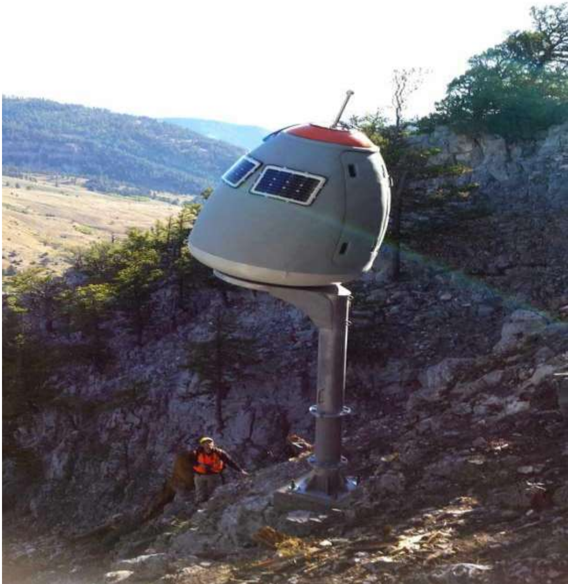
Figure 16. WYDOT's remotely operable, portable/helicopter deployable TAS O'Bellx® gas exploder, above US Route 189/191, in Hoback Canyon, Wyoming.
