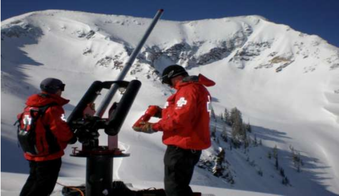
Figure 9. A compressed air launcher, Avalauncher®, being used in the Alta ski area, Utah, to deliver an explosive charge into avalanche starting zones.
