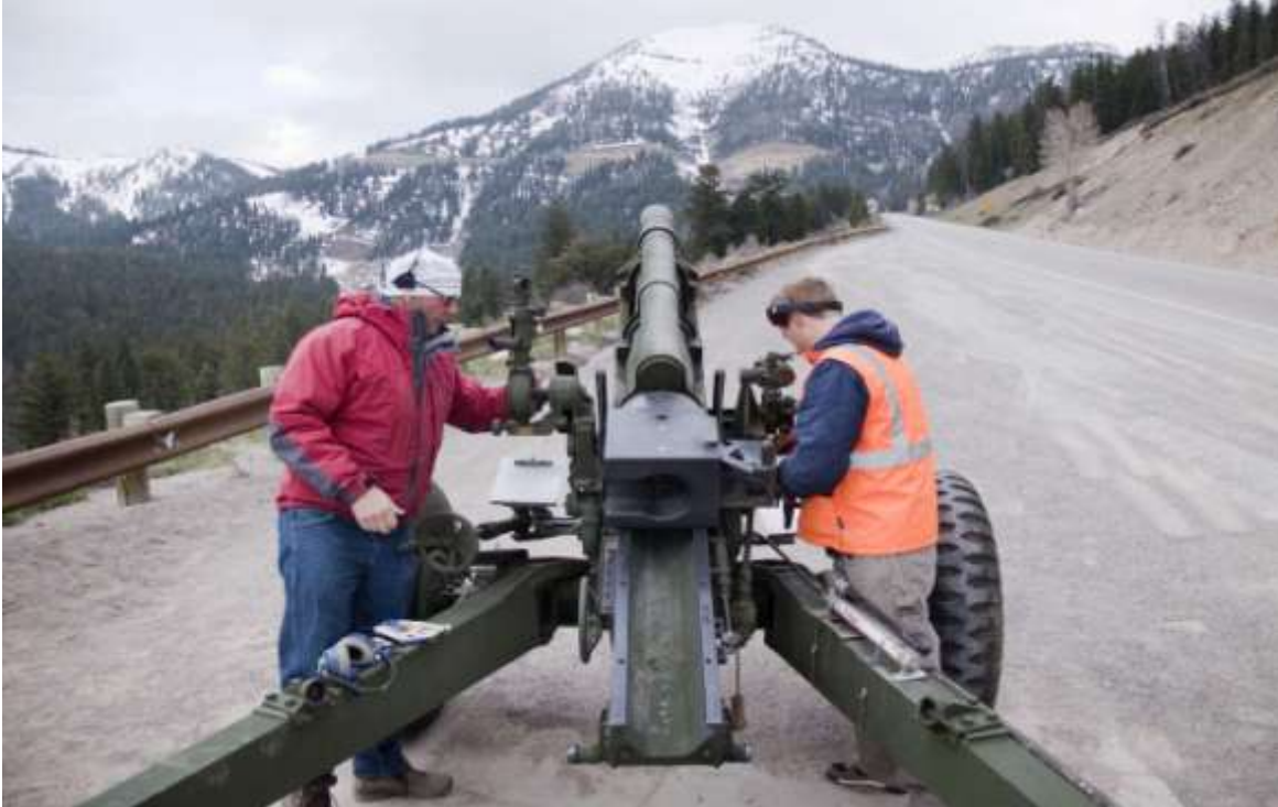
Figure 11. A military artillery weapon being used for active avalanche control by WYDOT personnel from a secure position on State Route 22, on Teton Pass, Wyoming.
