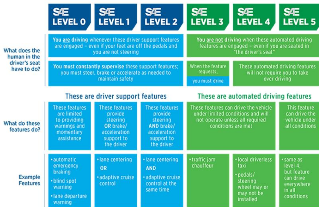
Figure 2. Summary of SAE Standard J3016 Levels of Driving Automation (Source: SAE, 2019)
