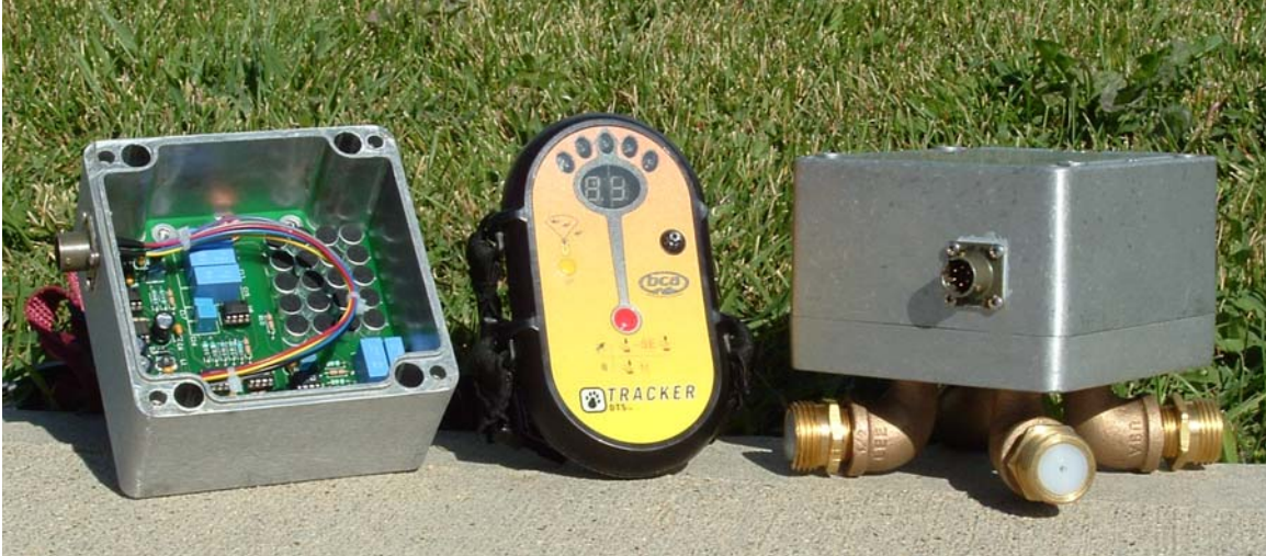
Figure 4. Prototype Infrasound Sensor Views with Avalanche Transceiver.
