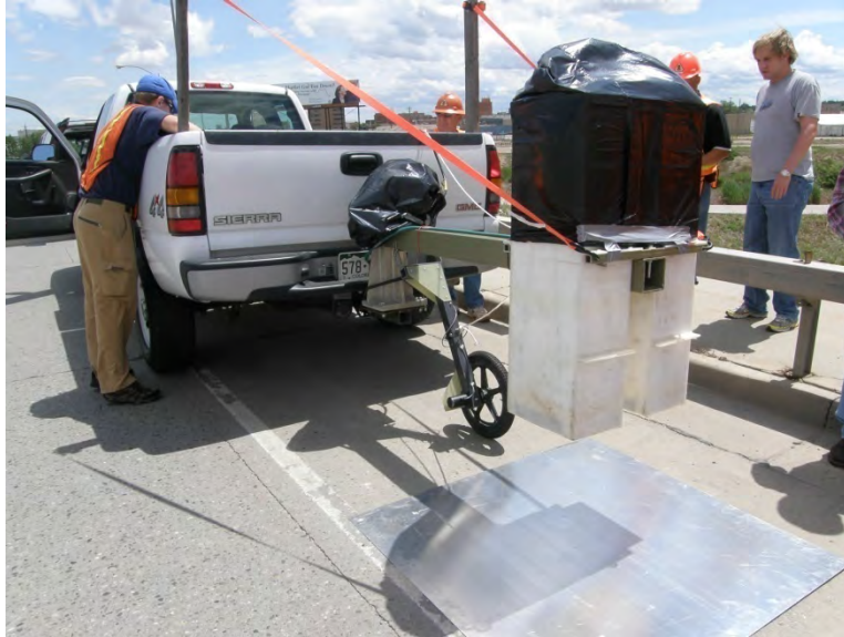
Figure 24: Truck-mounted GPR system.
