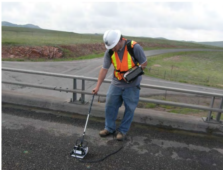
Figure 30: IDS Aladdin ground-coupled radar system.
