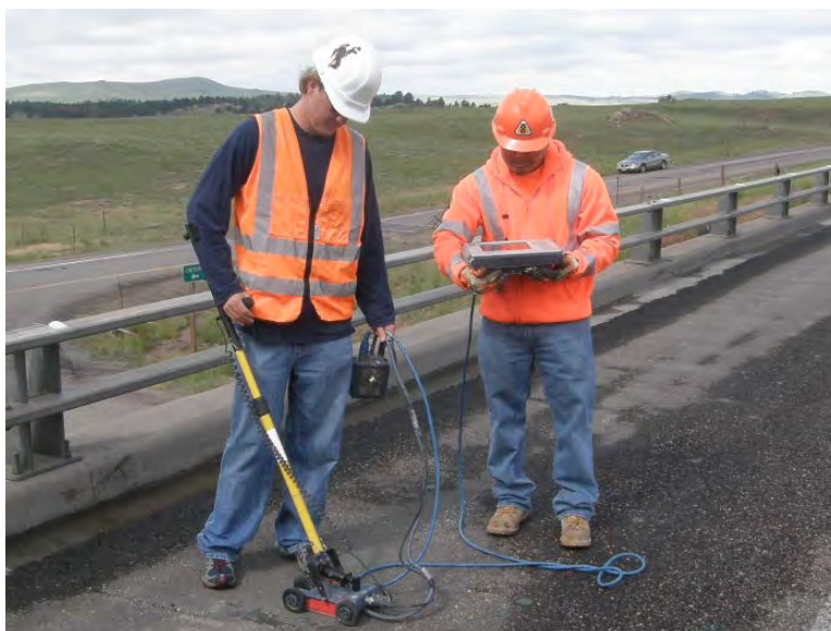
Figure 23: Ground-couple GPR system without cart.
