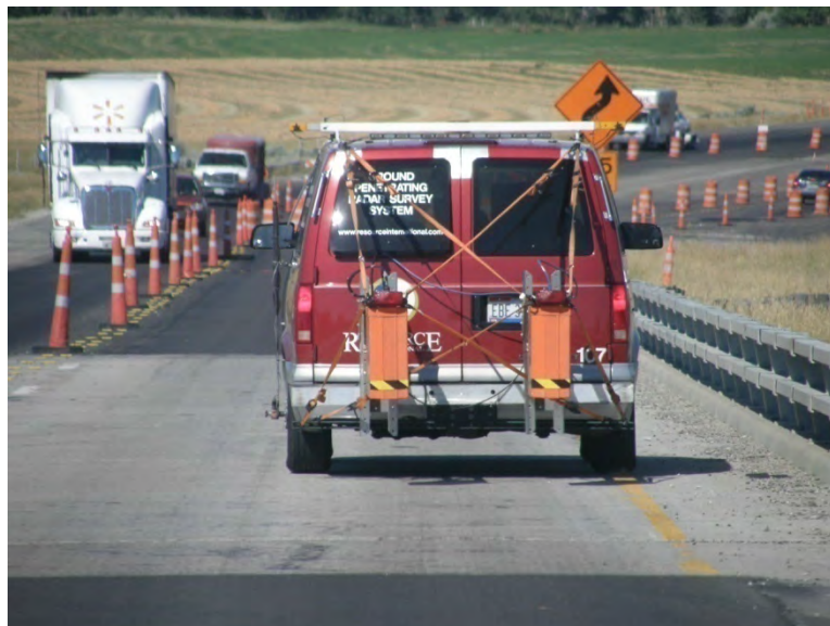
Figure 29: Rii's van-mounted system scanning the bridge.
