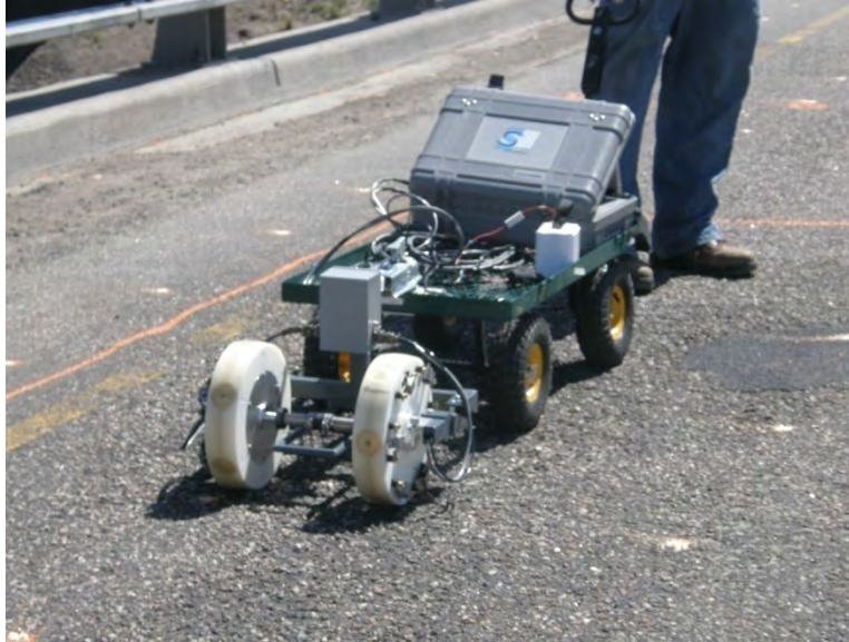
Figure 5: Olson Engineering's Impact Echo Bridge Scanner.
