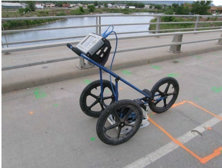
Figure 22: Ground-coupled GPR system.
