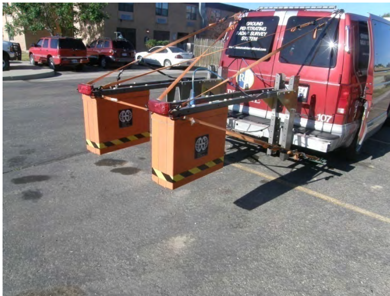
Figure 26: Radar apparatus on Rii's van.
