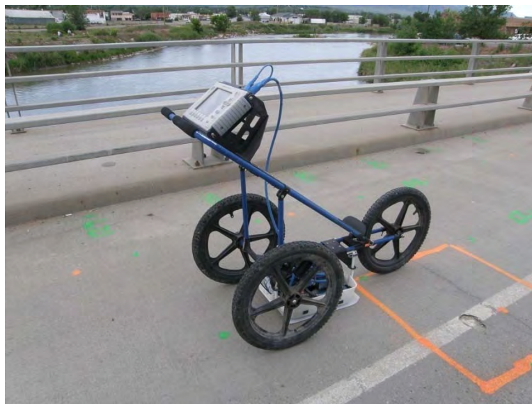
Figure 10: Typical GPR ground-coupled cart.
