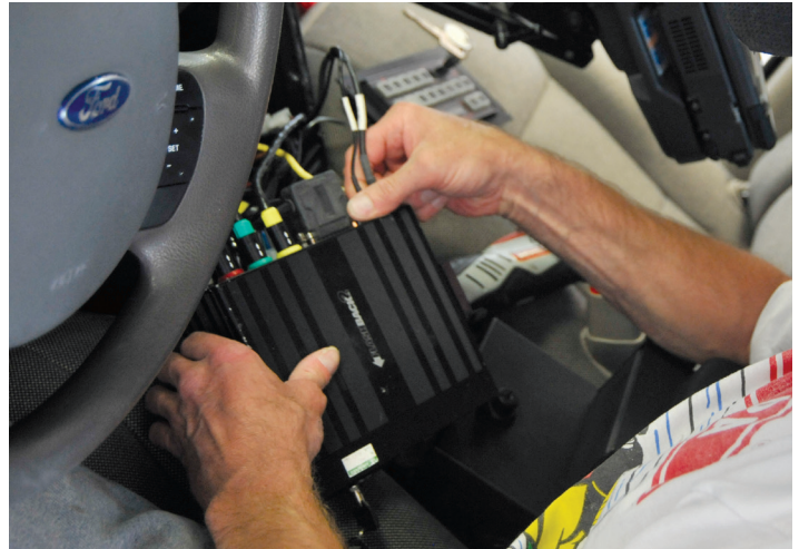
A telecom employee installing a WYOLink radio system in a WYDOT vehicle.
