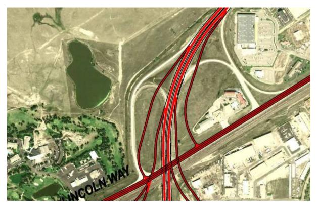
Alternative A1 replaces the current trumpet ramp design with a half diamond interchange using the existing I-25 under-crossing. Access to I-25 is limited to the SB I-25 off-ramp and NB I-25 on-ramp. These ramps are redesigned to 50 mph.
