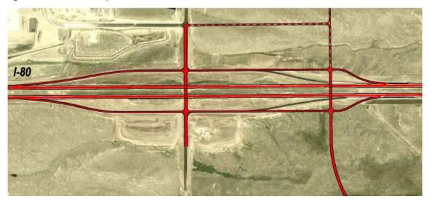
Alternative B2 consolidates the I-80/Lincolnway and I-80/Roundtop interchanges into a split diamond. The split diamond concept could ultimately have four traffic signals with two-lane, one-way CD roads connecting the ramps between the two service roads.
