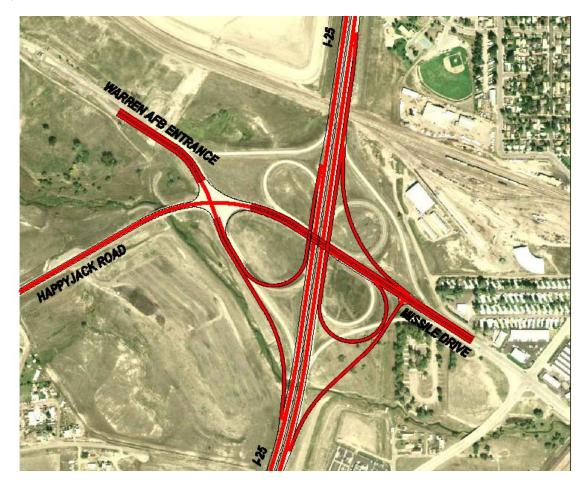
Alternative D2 converts the full cloverleaf to a two-loop PARCLO A/B interchange. Alternative D2 has two loops on the south side of Missile Drive to maintain a higher capacity for the SB to EB and the WB to NB movements. The loop ramps are designed at 30 mph and the directional ramps at 55 mph on and off I-25.
