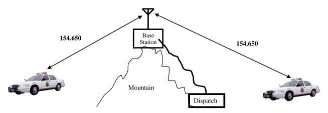
In this illustration, the dispatcher will be able to communicate with both patrol cars. However, with the mountains separating them, the two patrol cars will not be able to communicate with one another. The dispatcher will have to relay messages between the two cars.
