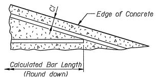
When bar lengths in a group or run require various lengths, rather than using a set, a uniform bar length may be employed to allow the lap between bars to be greater than the required minimum in order to facilitate fabrication and construction.
