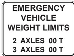
Regardless of how much of the total weight of a vehicle is actually on the bridge, the GVW must be equal or less than the limit next to the applicable vehicle. A blank indicates that vehicle is allowed to cross up to the legal GVW for that configuration.
