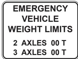
Regardless of how much of the total weight of a vehicle is actually on the bridge, the GVW must be equal or less than the limit next to the applicable vehicle. A blank indicates that vehicle is allowed to cross up to the legal GVW for that configuration.
