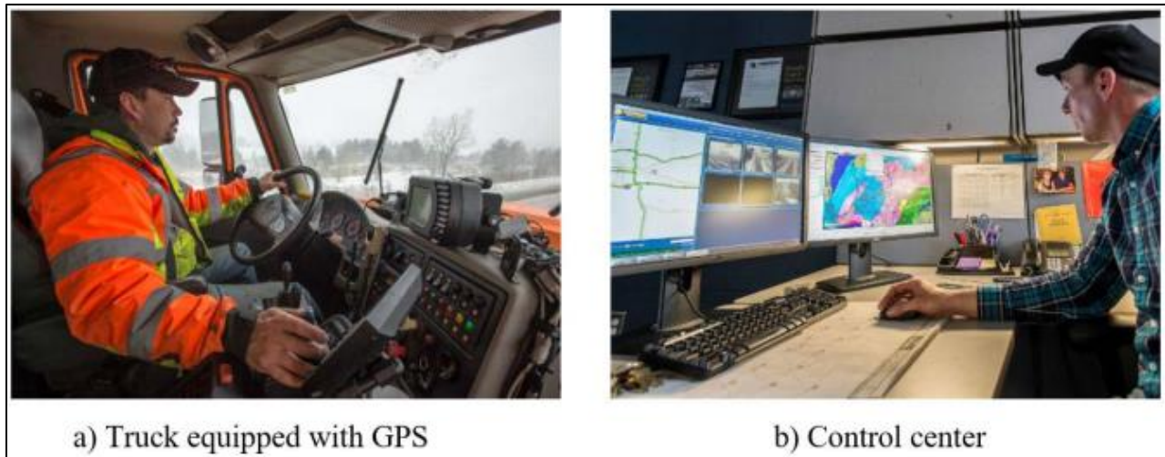
Figure 5: Automatic Vehicle Location (AVL) for Winter Maintenance Vehicles. (Source: Michigan DOT, 2018)
