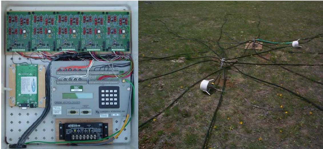
Figure 3. Remote Monitoring Node Instrumentation.
