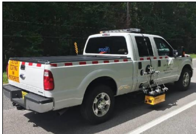
Figure 4: Typical mobile retroreflectivity unit installed in test vehicle.
