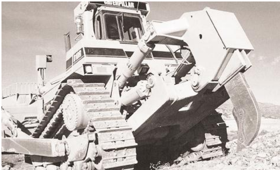
Figure 1. A Caterpillar bulldozer with a single shank (Caterpillar Inc., 2000)
