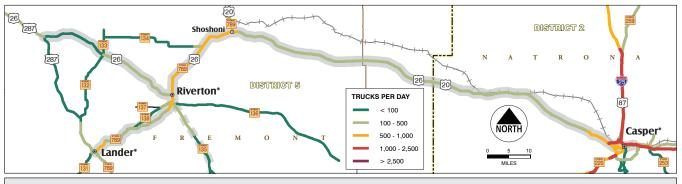
The truck traffic along most of SSC 10 averages 100 to 500 trucks per day. Truck traffic on some segments are in the range of 500 to 1,000 trucks per day and include WYO 789 northeast of Lander, US 26/WYO 789 between Riverton and Shoshoni, and west of Casper.
