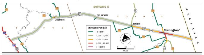
Most of SSC 16 from I-25 to the Nebraska state line averages less than 5,000 vehicles per day (vpd). US 26, from I-25 to US 85, averages 1,000 to 2,500 vpd with a short segment west of WYO 270 averaging 2,500 to 5,000 vpd. From US 85 to the Nebraska state line, US 26 averages 2,500 to 5,000 vpd increasing to 5,000 to 10,000 vpd for a short segment entering and exiting Torrington.
