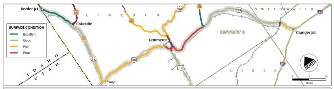
US 30 is rated as having surface conditions that are good/excellent for 68 percent of the corridor. Highway surface conditions closer to Border Junction, Kemmerer, and Granger are rated as Fair. Local routes WYO 233 and WYO 232 are rated as poor.
