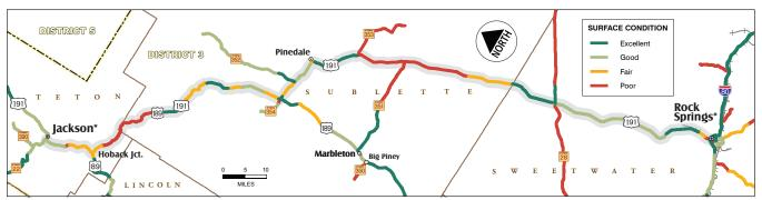
Nearly half of SSC 4 has pavement surface conditions that are rated good/excellent, including the segments from Rock Springs to the Sweetwater/Sublette county line and in the Pinedale area. Intermittent segments are rated fair, as shown. Segments with poor surface condition, approximately 28 percent of the corridor, include US 191 south of Pinedale and US 189/191 approaching Hoback Junction.
