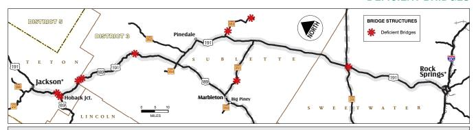
There are nine deficient bridges along SSC 4. Six of the nine bridges are located along US 191. Two of the bridges are located on WYO 353, and one bridge crosses the Green River on WYO 351 between US 191 and Marbleton. All deficient bridges visible in the map window are displayed, regardless of designation as SSC, Regional, or Local Routes.
