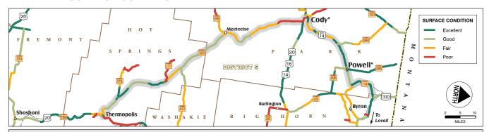
WY 120 is rated mostly good/excellent surface conditions from Thermopolis to Meeteetse. From Meeteetse to Cody, WY 120 is mostly rated fair to poor. From Cody to Powell along US 14A the surface conditions are mostly rated excellent, with intermittent areas where the surface conditions are rated fair. From Powell northeast to the junction with US 310 the surface conditions are rated mostly fair.
