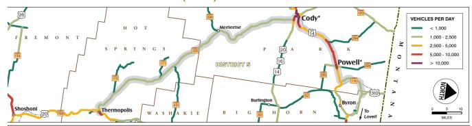
The majority of SSC 7, from Thermopolis to Cody along WYO 120, averages 1,000 to 2,500 vehicles per day (vpd). Just northeast of Cody, along US 14A, the AADT increases to 2,500 to 5,000 vpd and then 5,000 to 10,000 vpd from just southwest of WYO 294 to Powell. From Powell to the junction with US 310, US 14A carries less than 5,000 vpd.
