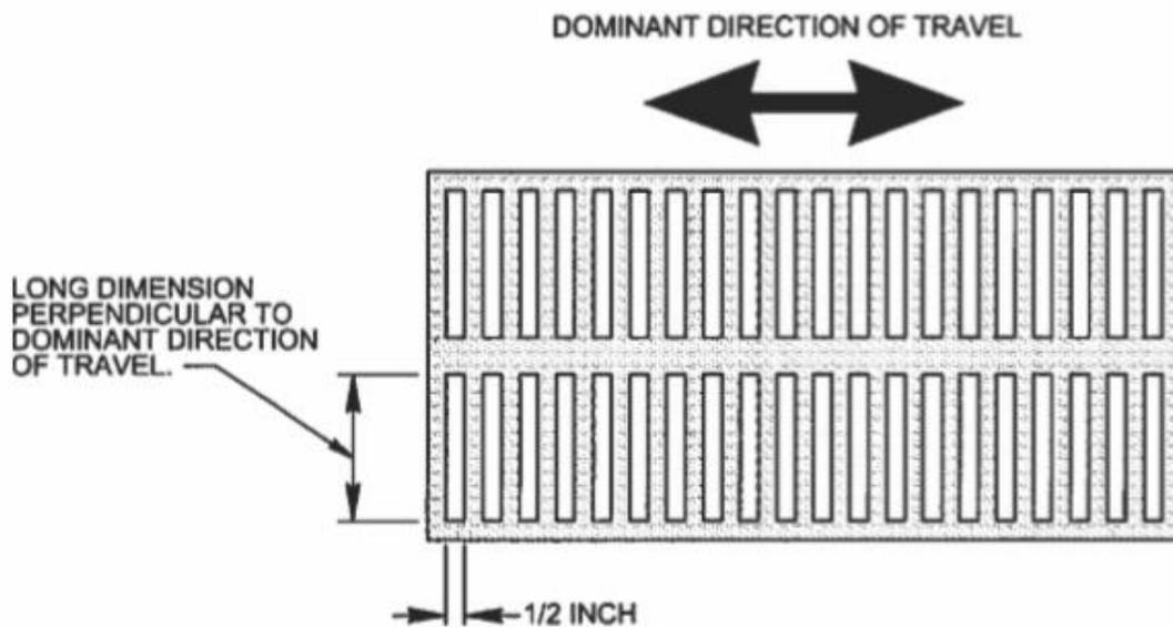
**Figure 3:** Horizontal Openings
