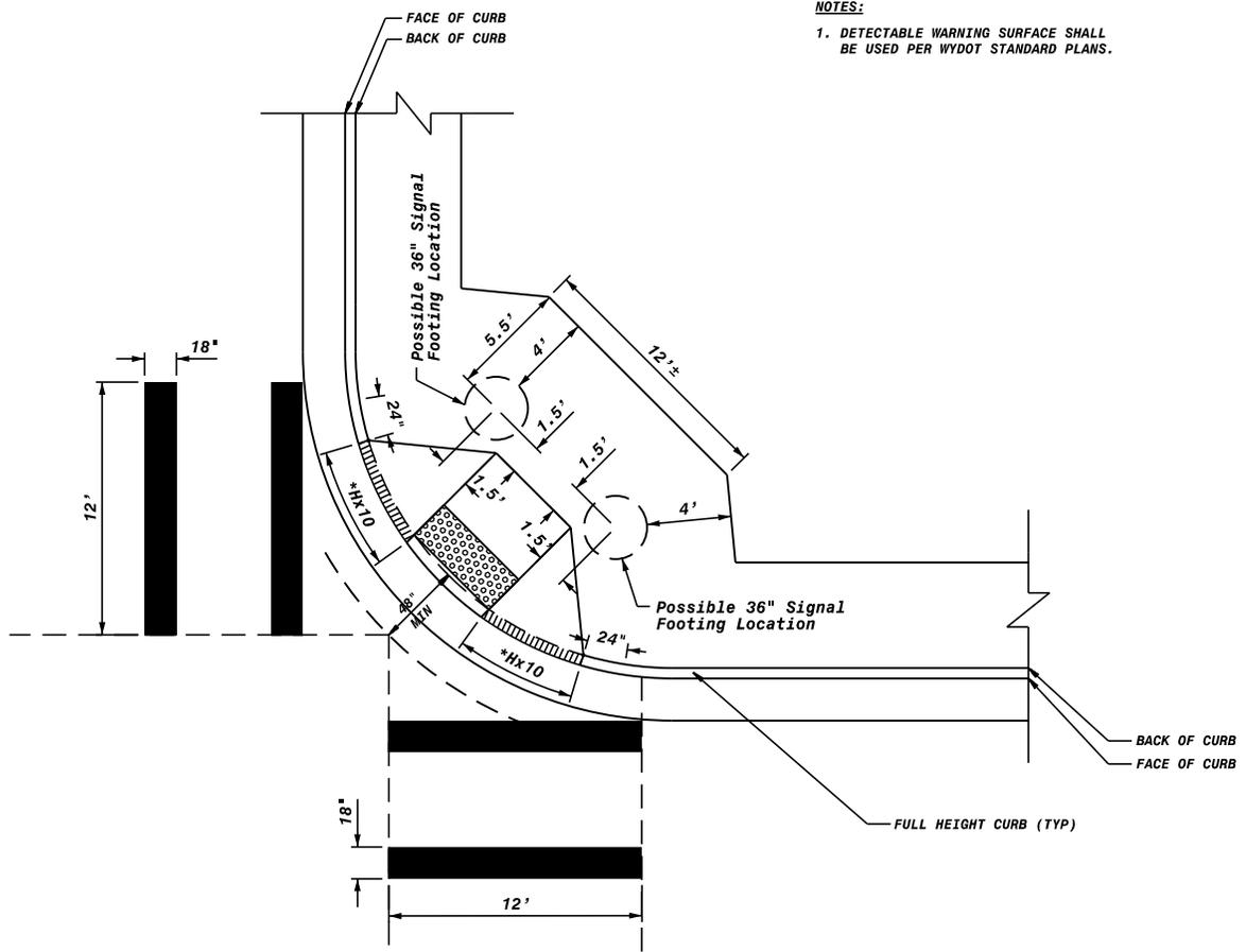
**APPLICATIONS FOR THIS DETAIL INCLUDE URBAN INTERSECTIONS WITH SHARP CURB RETURNS AND NARROW SIDEWALKS. PEDESTRIANS WILL ENTER THE INTERSECTION ON AN ANGLE. THE VISUALLY IMPAIRED DO NOT ADVOCATE DIAGONAL RAMPS BECAUSE IT IS REASONED THAT THE RAMP WILL DIRECT BLIND INDIVIDUALS INTO THE INTERSECTION. IF THIS RAMP IS APPLIED, AND ADJOINING SIDEWALK SHALL BE CONSTRUCTED OF 8" CONCRETE SINCE AUTOMOBILES AND TRUCKS MAY TRACK OVER THE CORNER. IT MAY BE APPLIED ON SIDEWALKS 5' WIDE OR GREATER.**
