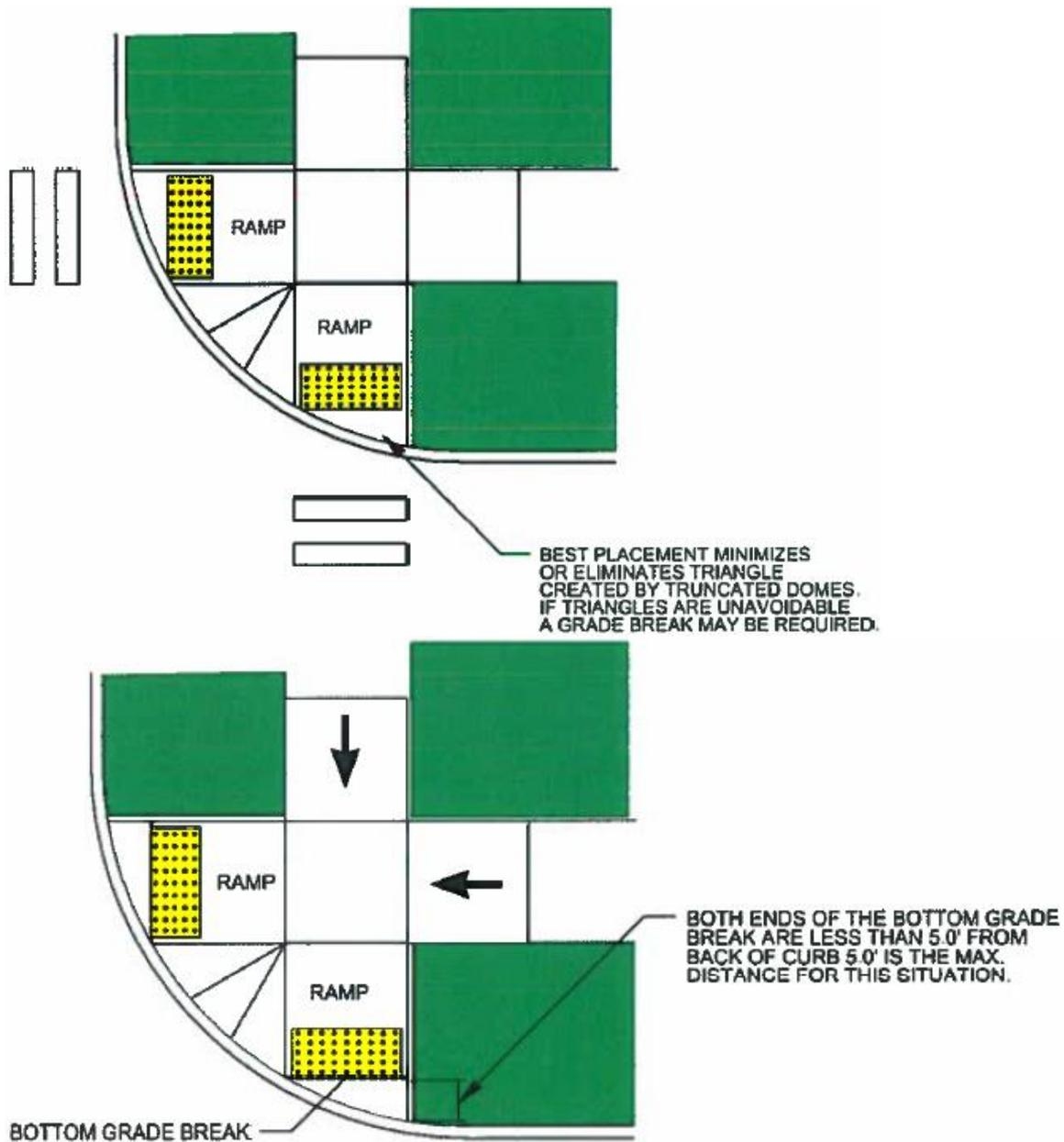
**Figure 7:** Detectable Warning Devices
