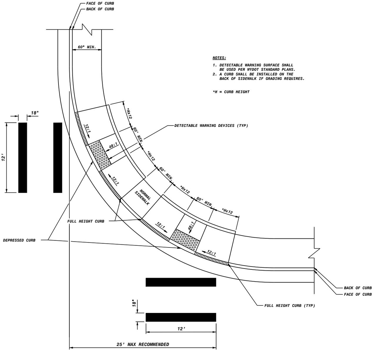
**APPLICATION FOR THIS DETAIL IS APPLIED TO URBAN OR SUBURBAN INTERSECTIONS WITH LARGE CURB RADI AND NARROW SIDEWALKS. IT DOES NOT ALLOW FOR PEDESTRIANS TO ENTER AN INTERSECTION AND CROSSWALK AT A RIGHT ANGLE. USE OF THIS DETAIL IS MOST APPROPRIATE AT SIGNALIZED INTERSECTIONS. SINCE THE SETBACK OF THE RAMP FROM THE CROSSING ROADWAY REQUIRES THAT THE STOP BAR BE INSTALLED FARTHER BACK THAN IS DESIRABLE FOR SAFE OPERATION AS A STOP-CONTROLLED INTERSECTION.**
