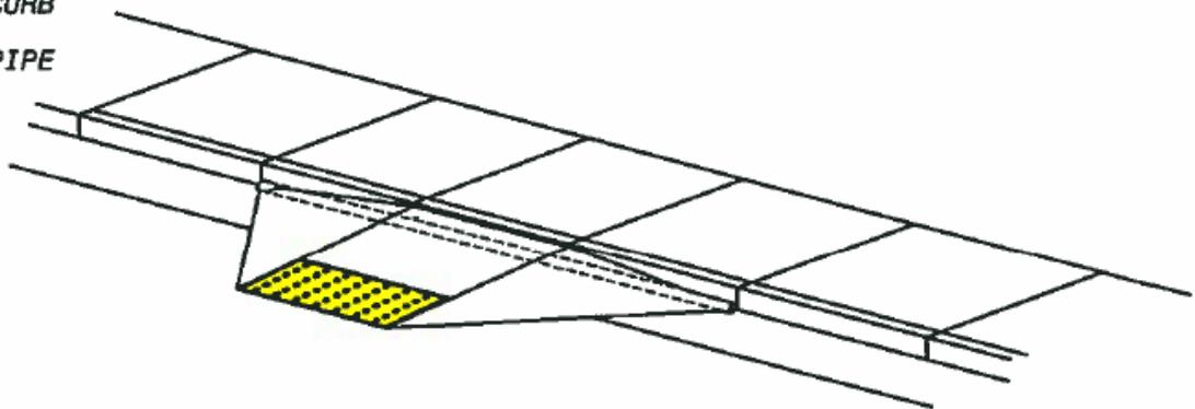
**Figure 13: Built-up Curb Ramp**
