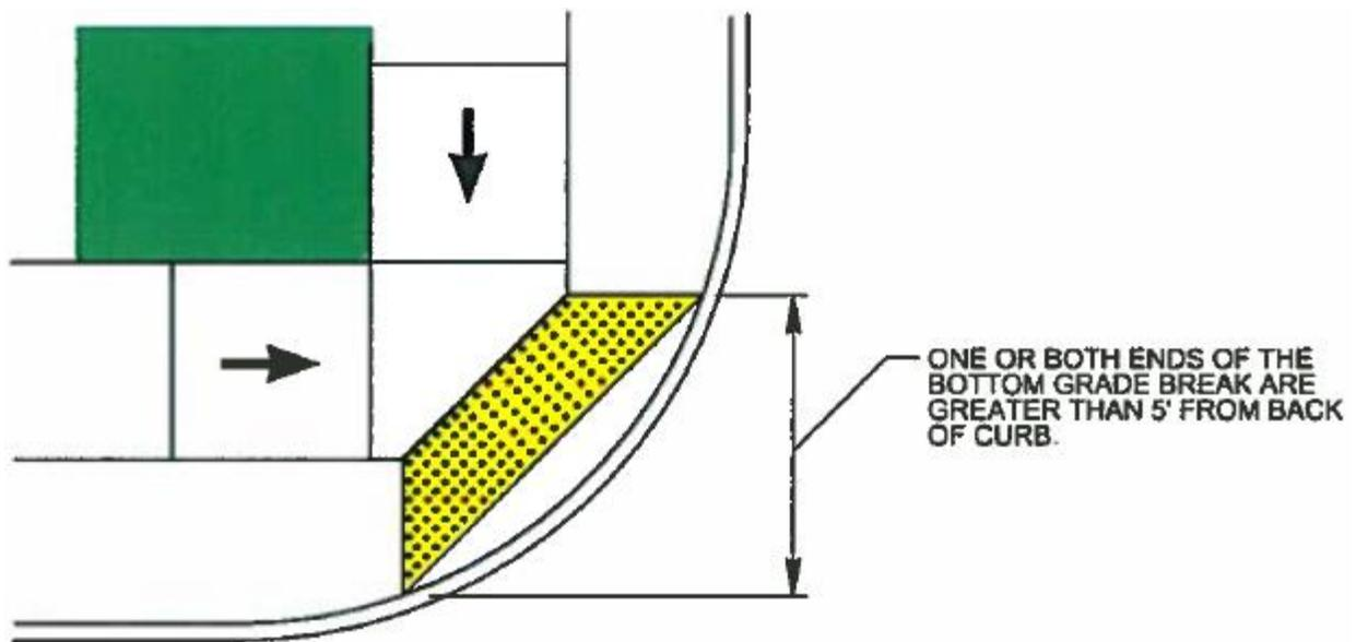
**Figure 7 (Cont.):** Detectable Warning Devices
