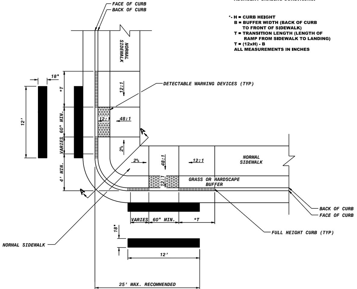
CURB OR CURB AND GUTTER AS CALLED FOR IN PLANS. MAX. CURB HEIGHT 4", MIN. 3" AS THERE MAY NOT BE ENOUGH DISTANCE TO TRANSITION BACK TO A 6" CURB.
