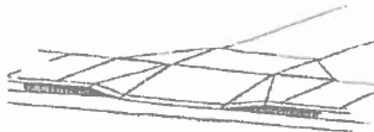
***Although parallel driveway crossings provide users with level landings, users continuing on the sidewalk are forced to negotiate two ramps.***
