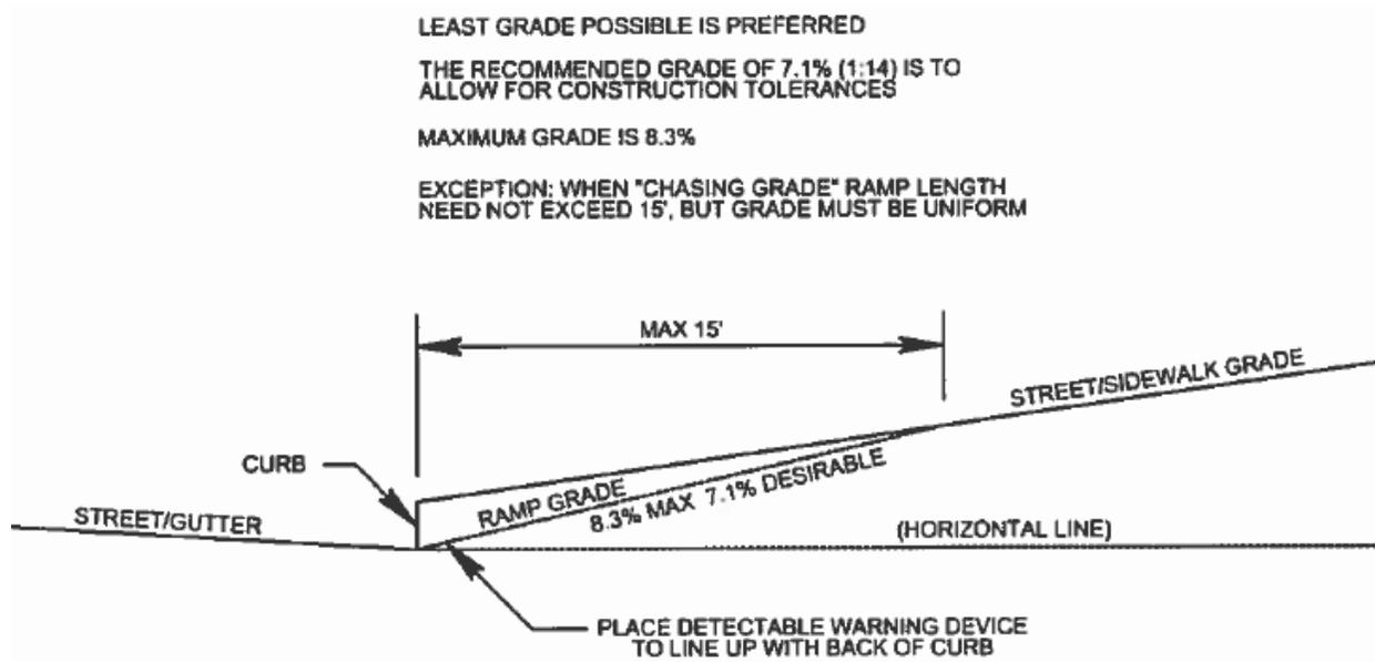
**Figure 26:** Curb Ramp Grade Retrofit
