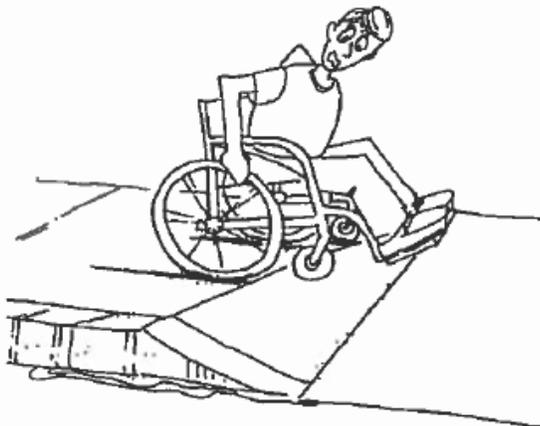
*When sidewalks have a planter strip, the ramp of the driveway does not interfere with a pedestrian's path of travel.*
