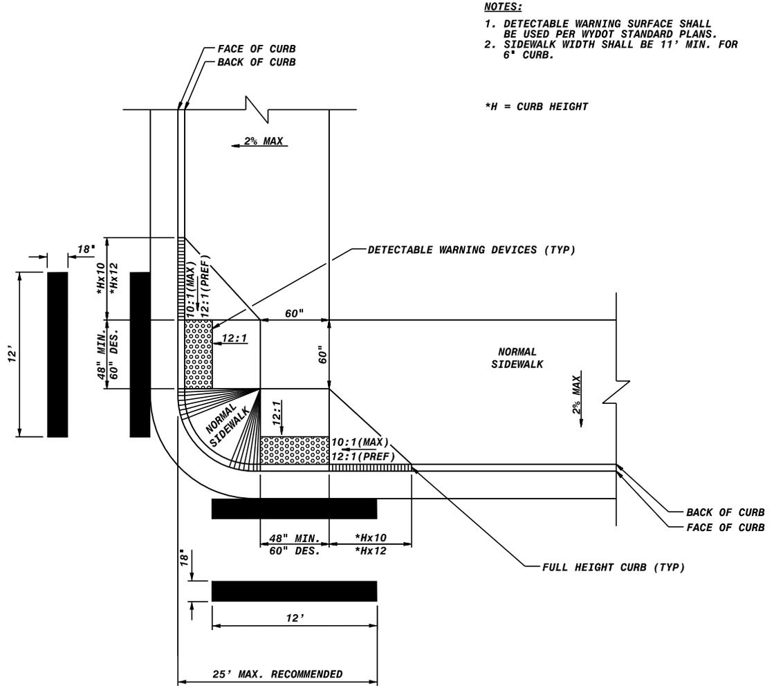
**APPLICATIONS FOR THIS DETAIL INCLUDE URBAN INTERSECTIONS WITH SHARP CURB RETURNS AND WIDE SIDEWALKS. IT ALLOWS FOR PEDESTRIANS TO ENTER AN INTERSECTION AND CROSSWALK AT A RIGHT ANGLE. FLARE SLOPES ARE SHOWN AS 10:1 MAXIMUM WITH 12:1 PREFERRED. THIS ALLOWS FOR CONSTRUCTION TOLERANCES AND SNOW AND ICY CONDITIONS.**
