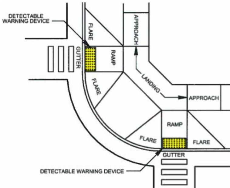
**Figure 6:** Standard Perpendicular Curb Ramp Components
