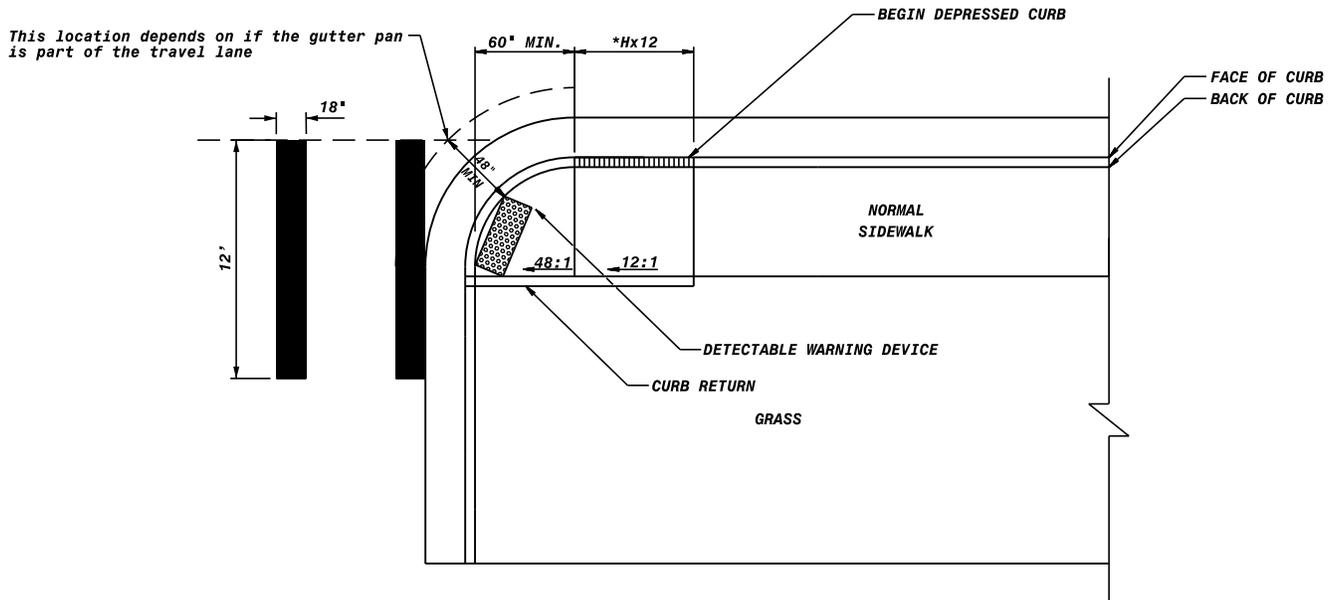
**APPLICATIONS FOR THIS DETAIL INCLUDE URBAN AND SUBURBAN INTERSECTIONS WITH SHARP CURB RETURNS AND SIDEWALKS IN ONE DIRECTION. PEDESTRIANS WILL ENTER THE INTERSECTION AT A RIGHT ANGLE. IT MAY BE APPLIED ON SIDEWALKS 5' WIDE OR GREATER.**
