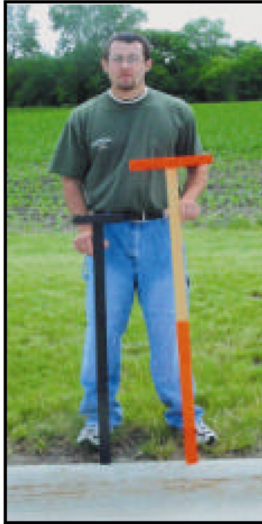
Figure 6-5 Example Sighting Rod (left) and Target Rod (right)
