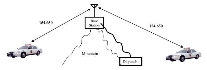
In this illustration, the dispatcher will be able to communicate with both patrol cars. However, with the mountains separating them, the two patrol cars will not be able to communicate with one another. The dispatcher will have to relay messages between the two cars.
