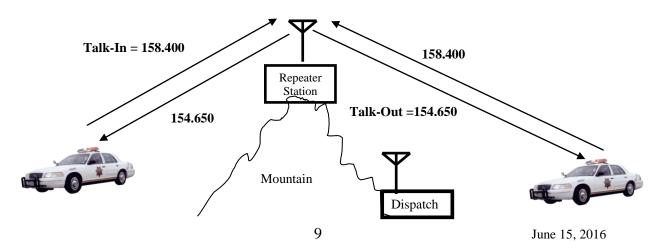
As illustrated above, the repeater receives the frequency being transmitted by the patrol cars (talk-in or repeater input) and the patrol cars receive the frequency being transmitted by the repeater (talk-out or repeater output).
