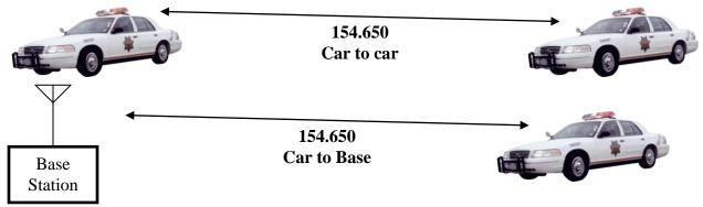
This mode of operation has the advantage of simplicity. Only the two radios are involved; no other technology is required. However, this mode has the disadvantage of limited operating range.
